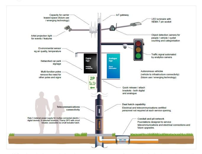
Multi-function poles in Maroochydore City Centre support a range of smart technologies that can be tested in a real world environment. Illustration is an excerpt from the <u>Smart Infrastructure Manual</u>.
